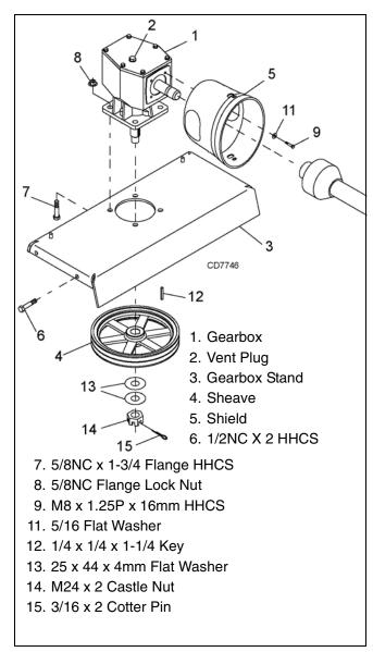
Figure 20. Gearbox Stand Assembly
